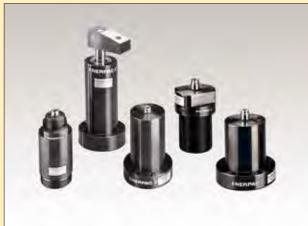
Enerpac Collet-Lok® cylinders are designed to mechanically hold the workpiece after hydraulic pressure is removed. Clamping capacities range from 4,4 to 37,8 kN.
