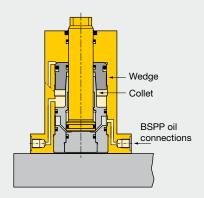
Hydraulic pressure pushes the collet up a wedge, locking the plunger in the clamping position.
