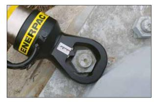
Heavily corroded and weathered nuts are quickly split and removed using a NS-Series Nut Splitter. Page:
