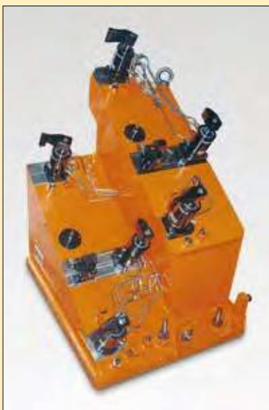
■ Fixture for machining exhaust manifolds.
