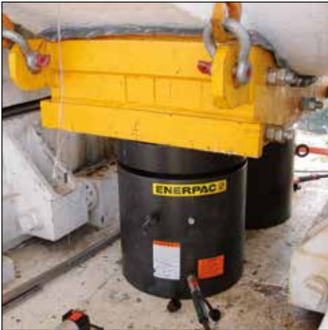
▲ Heavy lifting and foundation levelling. The lock nut provides mechanical load holding over a long period of time.
