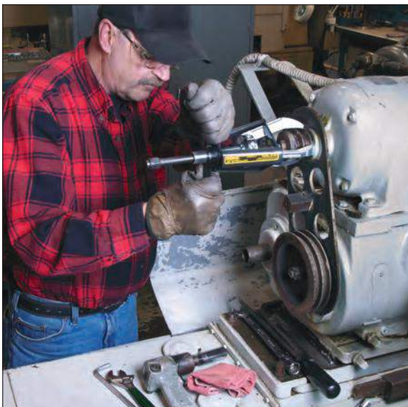
◀ Positioning an EP-104, 3-jaw puller on the drive pulley of an electric motor.
