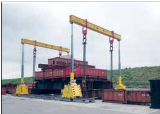
◀ SL-400 Gantry during load testing.
