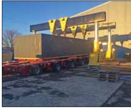
Hydraulic Boom Gantry Safely Transports 120 Ton Machine Bed
