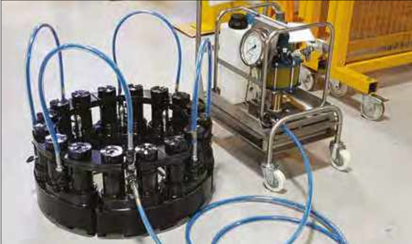
▲ Multi Stud Tensioning Set-Up.
