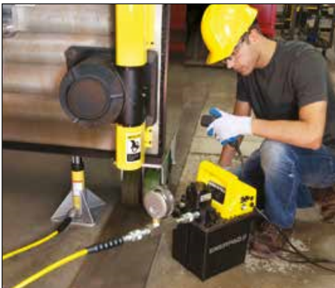
◀ The Remote Jog model (PEJ-Series) of the Submerged Pump simplifies maintenance on this machine.
