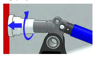
The TFA tools can be supplied with a Foot Extension that can be fixed to the adjustment leg to increase the effective leg length and therefore the range of application.
